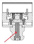
Socket Head Cap Screws DYNOGRIP-96: M10x1.5 x 40mm long
