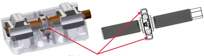
Slots allow movement to accommodate variation in material width
