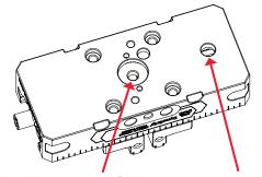
All 96 vises have a center ZPS hole: ø25 H6 hole with M10x1.5-6H fits Schunk:
